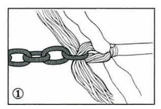
1. Apply a very snug Double Constrictor to the rope about 15-18 inches from the end. Separate the yarns into 4 equal-sized bundles and tape the ends. Pass 2 opposite bundles through link 1, in opposite directions. Draw up and fair, so that all yarns are taking an equal strain.
