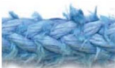
fig. 3 Severely abraded rope
