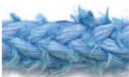
fig. 3 Severely abraded rope
