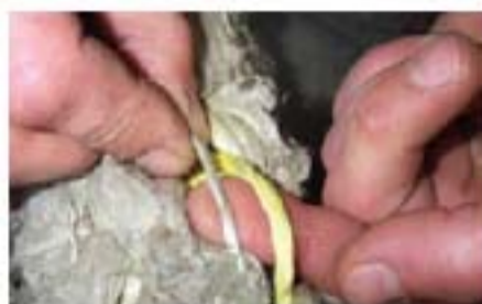
fig. 6 Compare surface yarns with internal yarns
