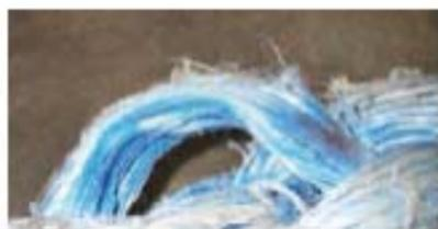
fig. 4 Inspect for internal abrasion
