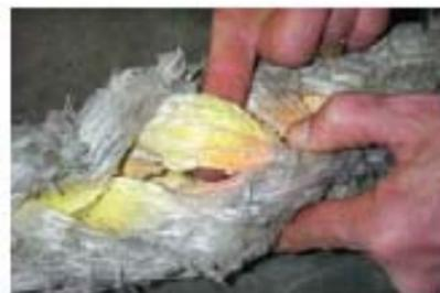
fig. 5 Inspect for internal abrasion
