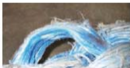
fig. 4 Inspect for internal abrasion
