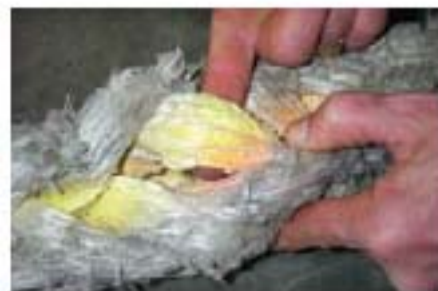
fig. 5 Inspect for internal abrasion
