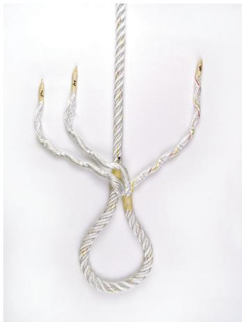
**Step #3** - To perform the first set of tucks, lay the strands out such that you have a left, middle, and right working strand. Then place the left and middle working strands across the rope just below the taped mark. (Fig 3) Tuck the middle strand under a strand on the standing part of the rope just beyond the taped mark.
