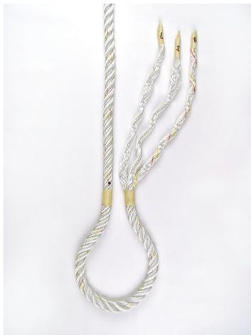
**Step #2** - To form the eye, bend the rope to form the desired eye size and mark with a temporary wrap of tape. This is done with the standing part of the rope in front of you, bending the tail of the rope from left to right. (note: bend following the natural bend of the rope so as not to put any twist into the eye or the splice). (Fig 2)
