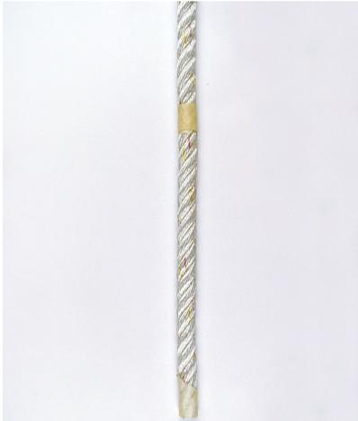
**Step #1** – To begin this splice, measure 14 crowns (or twists) from the end of the line [18 crowns for a tapered splice]. Mark this location with a temporary wrap of tape around the rope. Un-lay the rope up to the tape. Heat seal or tape the end of each individual working strands. (note: be careful that the strands do not untwist). (Fig 1)
