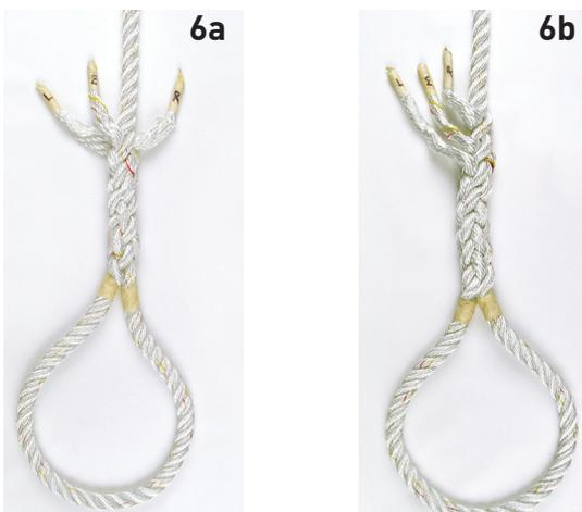
**Step #5** - Skip the step #5 if performing a standard splice. To perform a tapered splice make two additional tucks with one strand and one additional tuck with a second strand, leaving the third strand as is. (Fig 6b)
