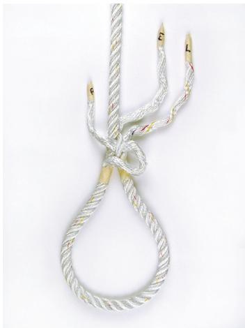
Take the right strand and tuck it under the strand just to the right of the one you raised for tucking the middle strand. Note: It is easier to do this if you first turn the rope over, as shown in photo) (Fig 5). Pull all three working strands snug (note: the two temporary tape marks should be aligning and forming your eye.) This completes the first set of tucks.
